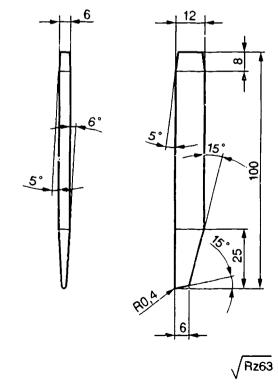
Sleeve for supporting gear shaft on adjusting response moment of overload protection: to be improvised
